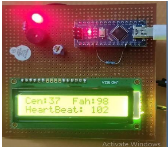
Figure3: practical implementation of monitoring system using Arduino.
